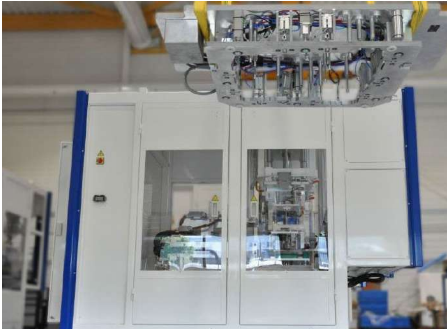
The upper and lower sides of the part are pushed towards the hot plate in order to transfer the heat energy, then separated and compressed for assembly.
